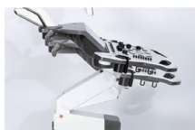
Lifting control panel
